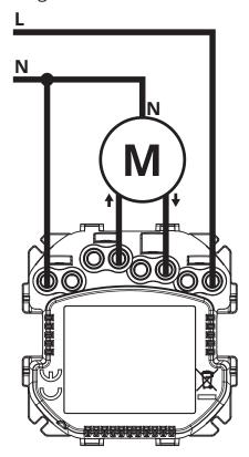
Diagram 1: Example connection with roller blind motor
