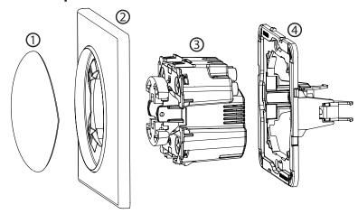
1 – switch button, 2 – cover plate, 3 – unit (device), 4 – mounting frame
